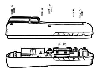
NOTE: If your meter does not work properly, check the fuses and batteries to make sure that they are still good and that they are properly inserted.
